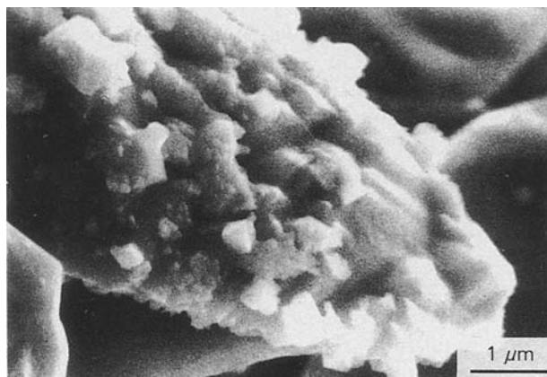
Figure 5 Scanning electron micrograph showing the presence of spinel and/or Al_4C_3 particles in an S10-composite sample cast above 735 °C.
